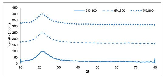
Figure 2. XRD analysis of SiO<sub>2</sub> on variations of HCl 3%, 5%, and 7%
