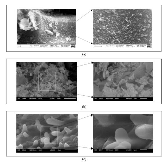
*Figure 1.* Results of SiO<sub>2</sub> morphological analysis of rice straw using SEM at variations of: (a) HCl 3%; (b) HCl 5%; and (c) HCl 7%.
